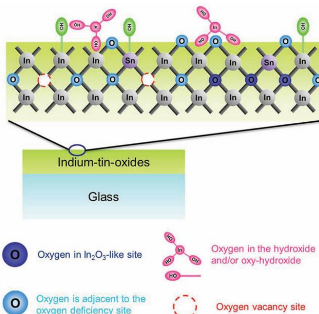
Figure 2. Schematic representation of an ITO surface model (Reprinted from Ref.2)
